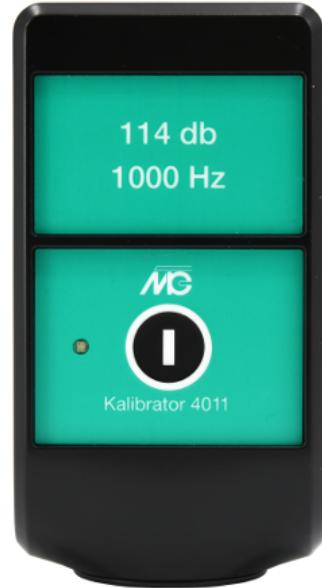
The 4011 is a sound calibrator conforming to IEC 60942 class 1 and ANSI S1.40 for the calibration and the verification of microphones and sound level meters. It generates a sound pressure level of 114 dB at a frequency of 1000 Hz for the verification of the calibration of sound level meters. Each sound calibrator is supplied with an individual calibration certificate.
